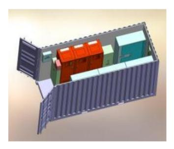
This Energy Storage equipment consists of 100kVA 3 phase bi-directional inverter and 400kWh of Lithium Manganese Cobalt Oxide batteries chosen for high cyclic life.
