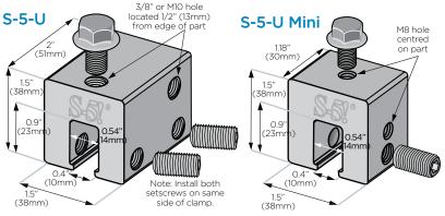
The strength of the S-5-U clamp is in its simple design. The patented set screws will dimple the metal seam material without penetrating it, leaving roof warranties intact.
