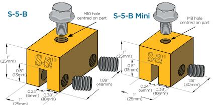
The strength of the S-5-B clamp is in its simple design. The patented set screws will dimple the metal seam material without penetrating it, leaving roof warranties intact.
