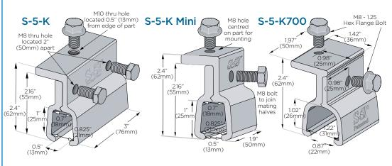
The S-5-K, S-5-K Mini and S-5-K700 clamps are each supplied with the hardware shown above. The S-5-K, S-5-K Mini and S-5-K700 clamps are compatible with most common roofing materials excluding Copper. All included hardware is manufactured from 300 Series Stainless Steel. Please visit www.S-5.com for more information including CAD details, metallurgical compatibilities and specifications.
