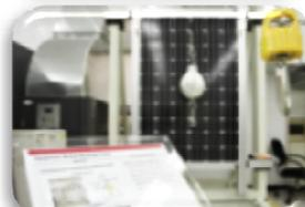
Impact Fracture Test
