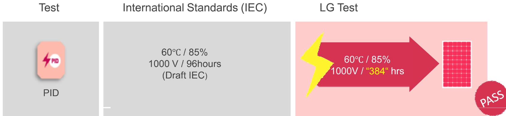
\* Potential Induced Degradation is a power degradation from exposure to High Voltage Stress.
