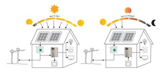
\* If at any time there is a grid failure the system can backup the loads to the set depth of discharge
