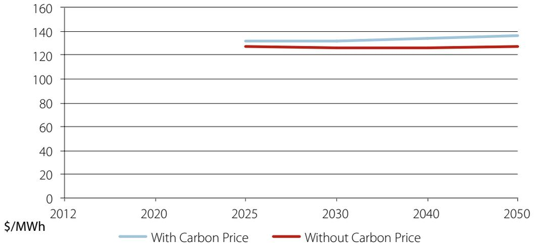
Table 4.14: Oxy combustion pulverised coal supercritical plant based on bituminous coal, LCOE, NSW
