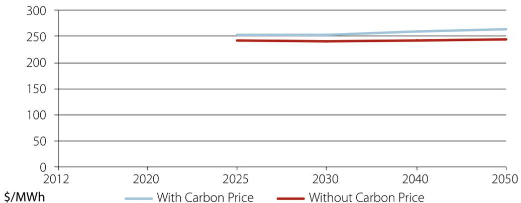
Table 4.5: Direct injection coal engine based on brown coal, LCOE, Victoria
