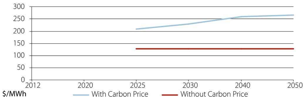
Table 4.15: Oxy combustion pulverised coal supercritical plant based on bituminous coal with CCS, LCOE, NSW
