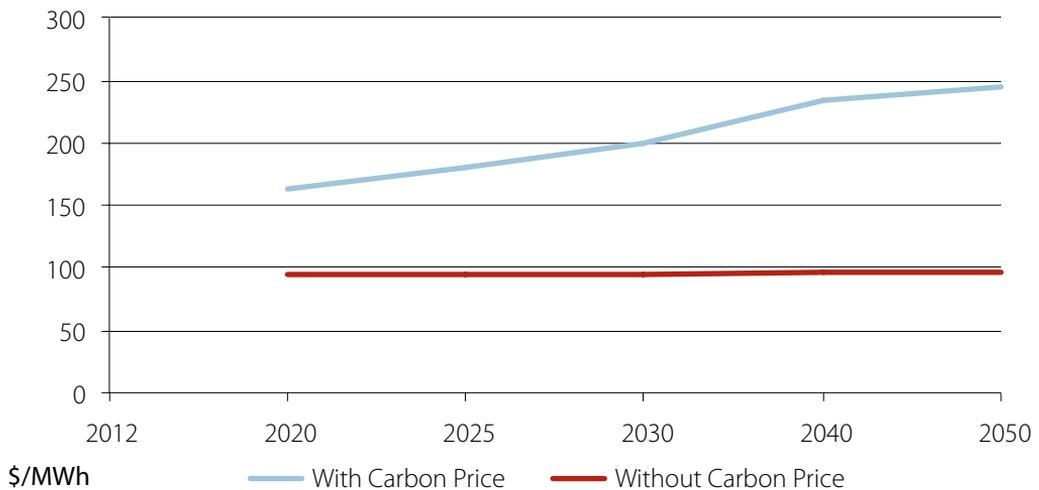
Table 4.7: Pulverised coal supercritical plant based on brown coal with post-combustion CCS, LCOE, Victoria
