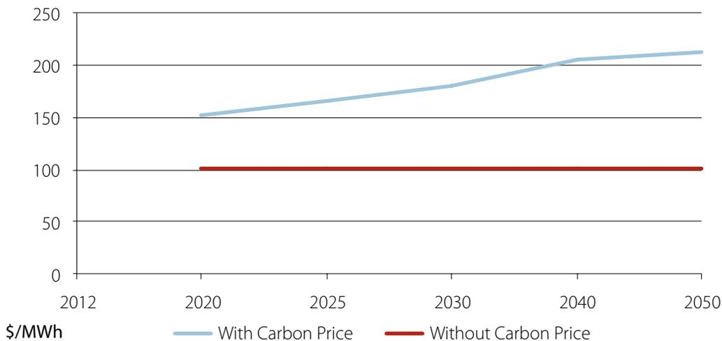
Table 4.11: Pulverised coal supercritical plant based on bituminous coal with CCS, LCOE, NSW
