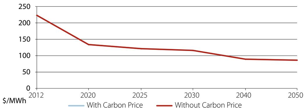
Table 4.27: Solar photovoltaic - single axis tracking, LCOE, NSW
