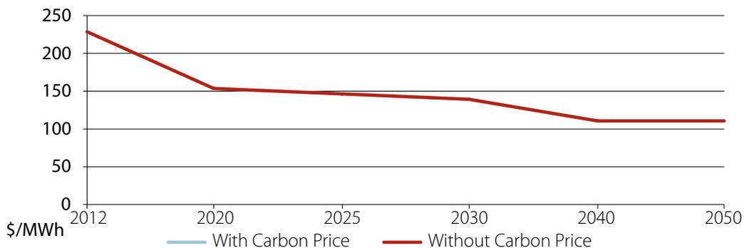
Table 4.28: Solar photovoltaic - dual axis tracking, LCOE, NSW
