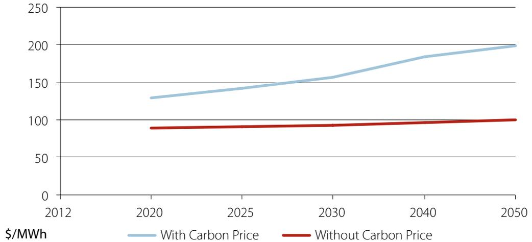
Table 4.6: Pulverised coal supercritical plant based on brown coal, LCOE, Victoria
