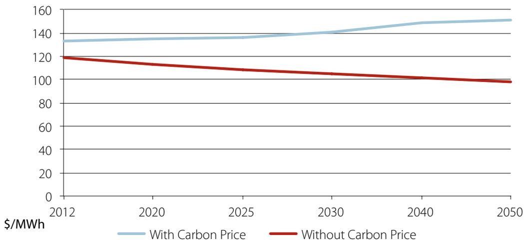
Table 4.18: Combined cycle plant with post combustion CCS, LCOE, NSW
