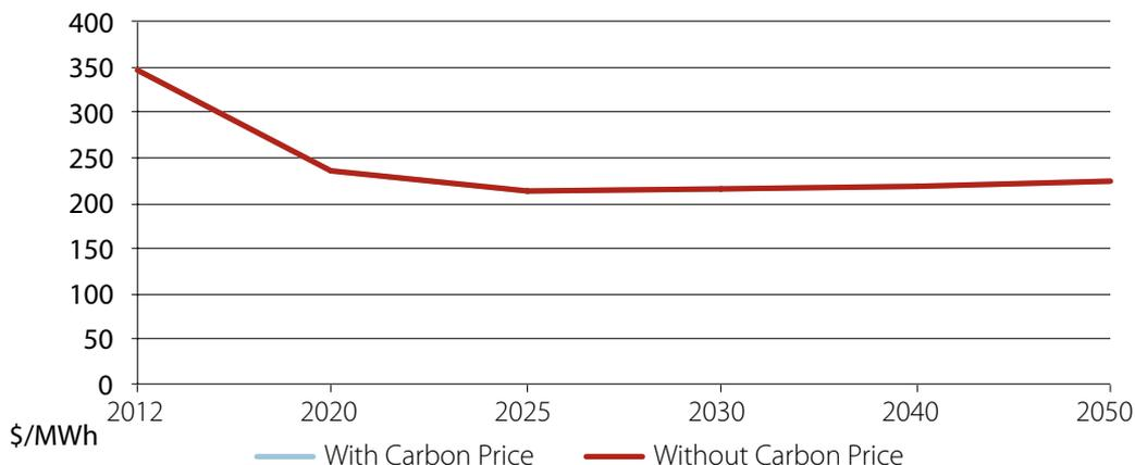
Table 4.22: Solar thermal plant using parabolic trough technology with storage, LCOE, NSW
