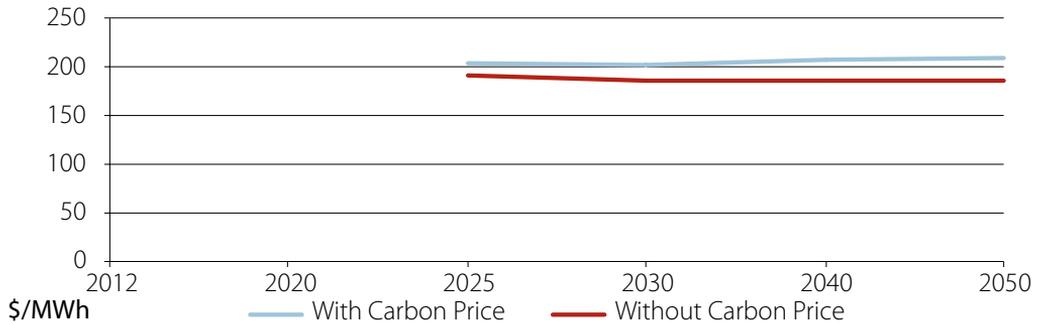
Table 4.8: Pulverised coal subcritical plant based on brown coal with retrofit post-combustion CCS, LCOE, Victoria
