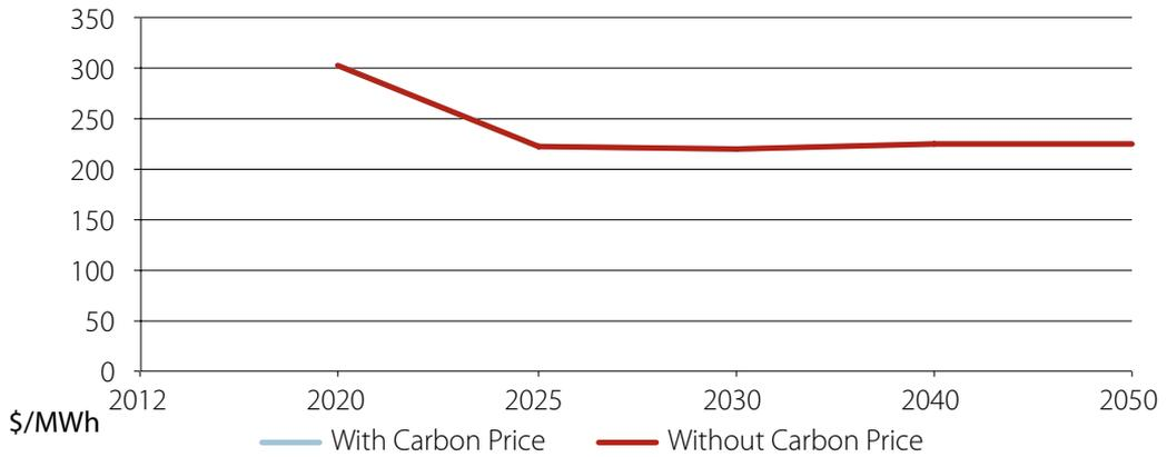
Table 4.32: Geothermal - hot sedimentary aquifer, LCOE, NSW
