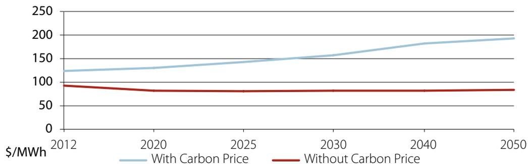
Table 4.40: ISCC; parabolic trough with combined cycle gas, LCOE, NSW
