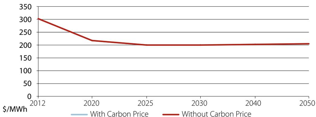
Table 4.25: Solar thermal plant using central receiver technology with storage, LCOE, NSW
