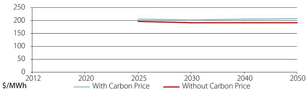
Table 4.12: Pulverised coal subcritical plant based on bituminous coal with retrofit post-combustion CCS, LCOE, NSW
