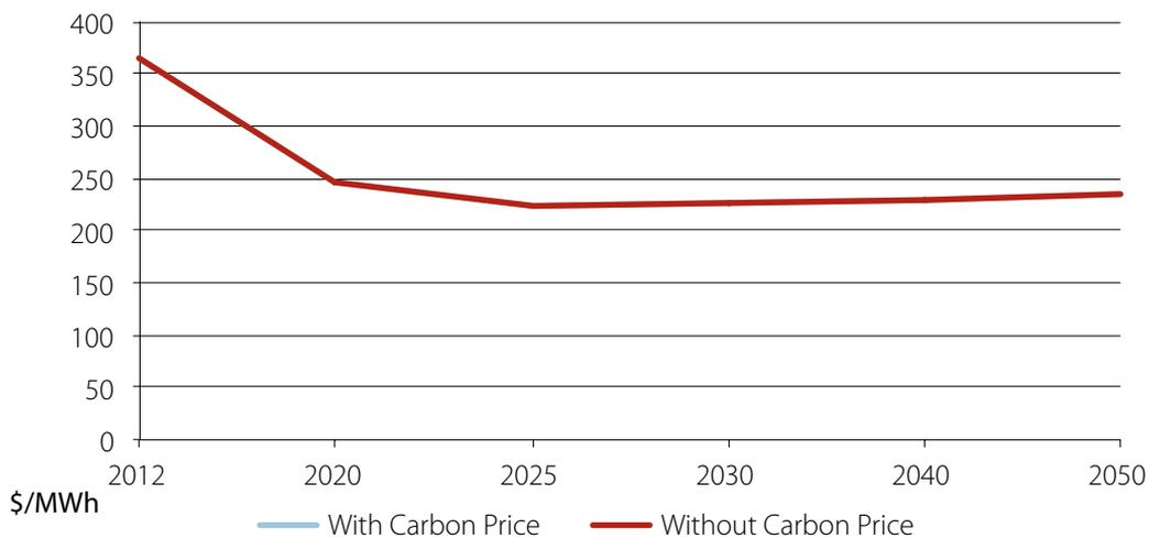
Table 4.21: Solar thermal plant using parabolic trough technology w/o storage, LCOE, NSW
