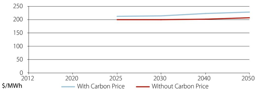
Table 4.3: IGCC plant based on bituminous coal, LCOE, NSW
