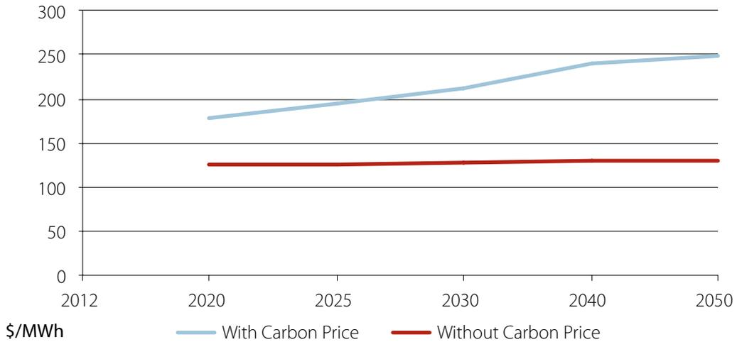
Table 4.4: IGCC plant based on bituminous coal with CCS, LCOE, NSW
