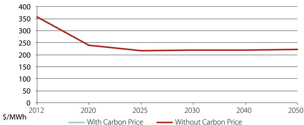
Table 4.24: Solar thermal plant using central receiver technology w/o storage, LCOE, NSW
