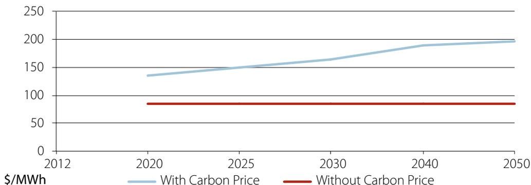
Table 4.10: Pulverised coal supercritical plant based on bituminous coal, LCOE, SWIS
