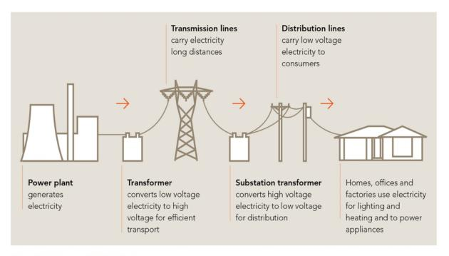
Figure 3.1 Transport of Electricity
