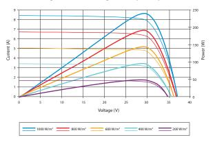
Exellent performance under weak light conditions: at an irradiation intensity of 200 W/m<sup>2</sup> (AM 1.5, 25 °C), 96% or higher of the STC efficiency (1000 W/m<sup>2</sup>) is achieved
