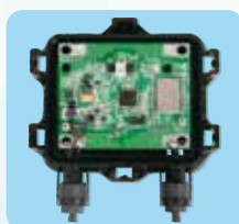
PV数据采集器 PV Data acquisition system
