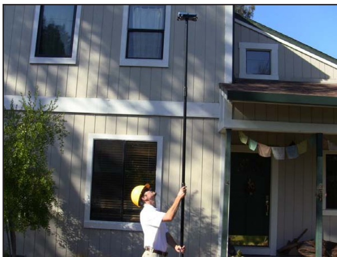
Extension kit enables rooftop measurements from ground level.
